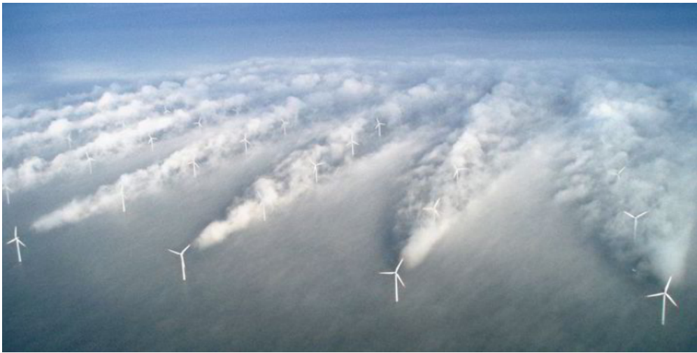
Figure 5: Illustration of the wake effect in wind power plants (Snieckus, 2019)
